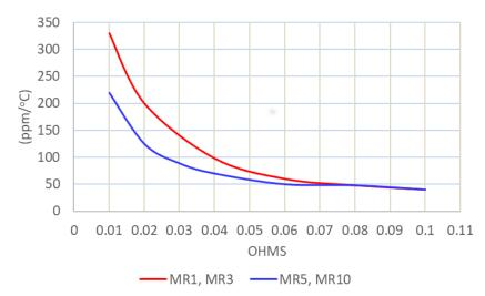
Low Resistance Value Resistor - Molded 2 and 4 Leads
