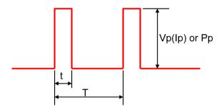
Where: Vp: Pulse limiting voltage (V)
