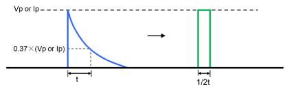
2. Damping oscillation wave with time constant of envelope "t" → Square wave
