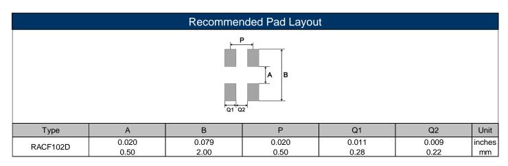
Concave Termination Chip Resistor Array
