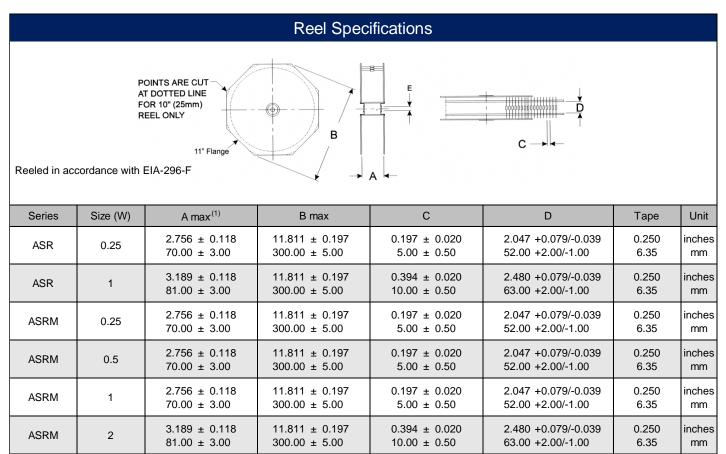
Dimension "E' This is a non-critic dimension that does not have a tolerance in the standard.
