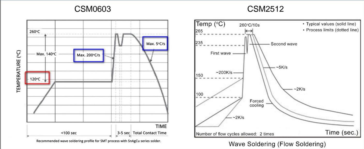
**Recommended Resistor Reflow Profile**
