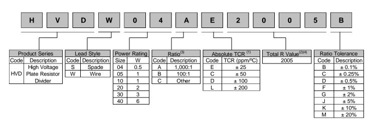
Note (1): TCR tracking typically < 25% of the absolut TCR to a minimum of 10 ppm/°C
