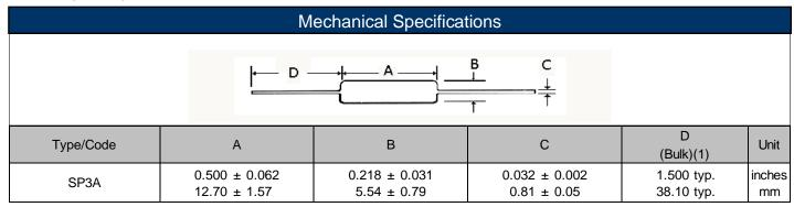
(1) See Packaging Specifications for lead length dimension for tape and reel packaged product Operating Temperature: -55°C to + 350°C
