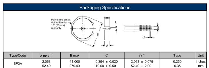
Dimension "E": This is a non-critical dimension that does not have a tolerance in the standard.
