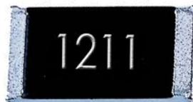
The nominal resistance is marked on the surface of the overcoating with the use of four-digit markings.
