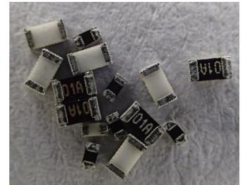
The RTAN series from Stackpole is a tantalum nitride thin film chip resistor that withstands biased humidity testing at 85 °C, 85% relative humidity, 10% rated power with very little resistance shift. In addition, the RTAN anti-sulfur materials and design is such that it will pass the rigorous ANSI/EIA-977 (method A) standard sulfur test with minimal resistance shift.
