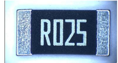
The CSRF2512 is rated at 2W and is available in resistance values from 2 milliohm up to 560 milliohm. Pricing for the CSRF2512 is around \$0.30 each in full package quantities. Contact Stackpole or one of our franchised distribution partners for specific or volume pricing. Many popular values are currently in stock.
