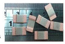
offers power ratings up to a 10W rated, 5930 size with TCR as low as 50 ppm, and a raised element to improve the thermal footprint of the device and decrease PCB and terminal temperature. Resistance values as low as 0.2 milliohm ensure the high efficiency sensing in a surface mountable package. The allmetal construction also provides very high pulse withstanding superior to that of film or foil on ceramic sense resistor types.
