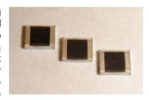
down to only 1%. Stackpole's CSRT current sense resistors feature tolerances down to 0.5% and TCR of 50 or 100 ppm depending on value and are AEC-Q200 compliant. In addition, the CSRT offers high power handling with a 2512 size chip rated up to 3.5W.
