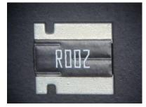
excellent TCR down to  $\pm 50$  ppm and resistance tolerance down to  $\pm 0.5\%$  for exceptional precision. The CSSK is available in resistance values from 0.5 to 6 milliohm making it able so sense currents of over 77 amps.
